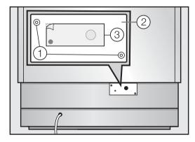
The slot for the RemoteVision module is located in the lower area of the back of your appliance.
